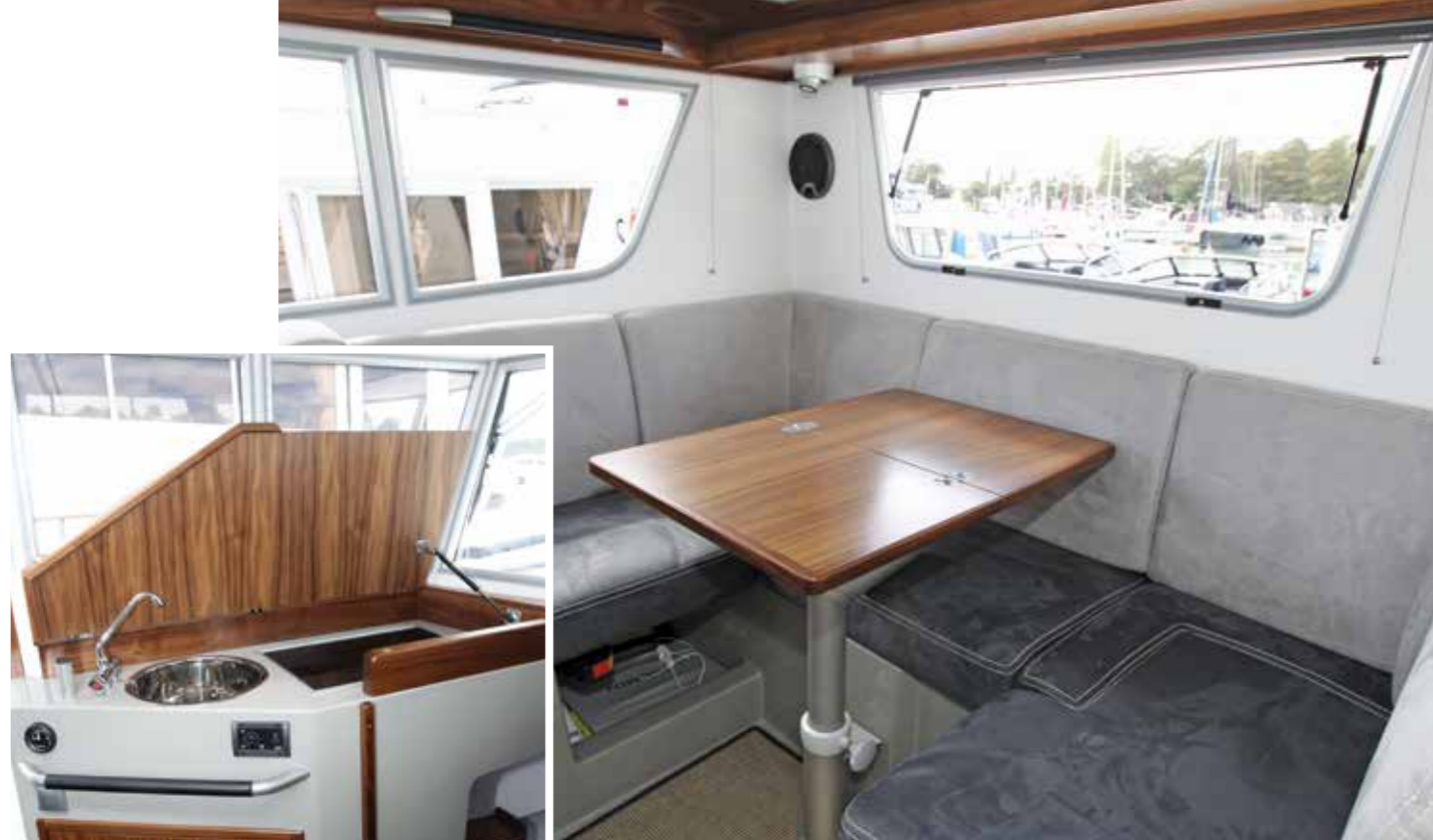
The galley and dinette in the wheelhouse separates the two double cabins at either end
